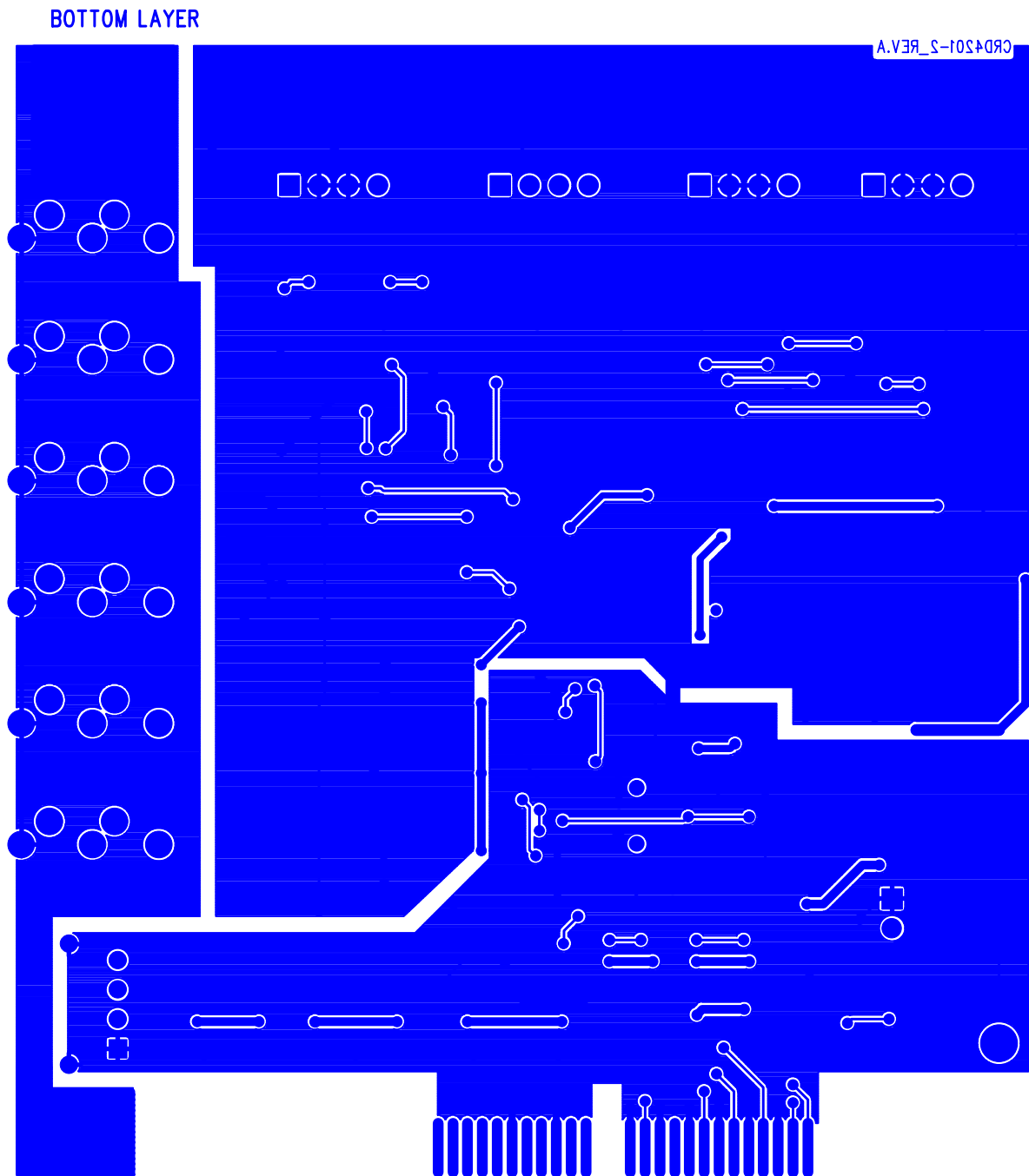
Figure 10. PCB Layout: Bottom Layer
